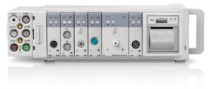
Z02 has a C30/C31 slot, 10 module slots, and a 48mm thermal printer slot; plug-and-play, flexible and extensible.
